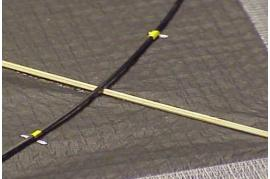
25. Place the kite face down on your work surface with the nose pointed toward you. Use the marks indicating the upper bridle connection points that you marked on the bow to mark kite skin. If you use bridle stops, like in the photo, use the edge of the stop closest to the bow tip as a guide for marking the skin.
