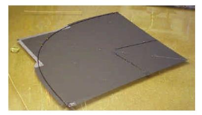
15. Raise the bow off the kite skin by placing a pen or other object under the bow near the bow/spine cross point. Apply glue to the bow and the bow hem area on both sides of the kite. Let it dry for a few minutes. If you're concerned about the exposed glued surfaces of the bow and skin touching each other before you are ready for them to, place a piece of waxed paper between the skin and bow. The waxed paper will be placed on wet glue.
