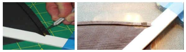
14. Lift up this tab you just created and wrap it around the bow. Do the same for the other side. Then remove the bow setter and fold over the remaining tab at the tip of the bow.
