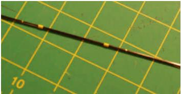
If you are using bridle stops, slide the stops near the center of the bow, place a drop of CA glue on the mark you made and slide one of the stops through the glue and align the edge of the stop closest to the bow tip with the mark. Do the same for the other stop.
