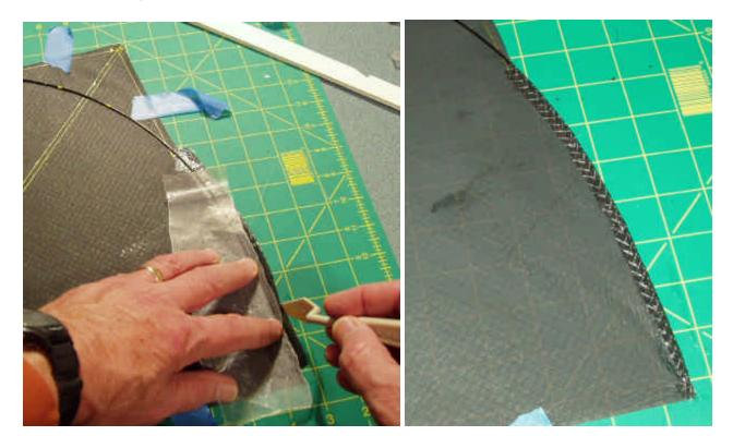
18. Although I don't show the waxed paper in the following photos, using it while installing the spine makes the job easier. Lay a small piece of waxed paper on the exposed spine glue line near the nose area and under the bow. Lift the bow near the bow/spine cross point enough to allow the spine to fit underneath it. Slide the spine under the bow keeping the tail end of the spine above
