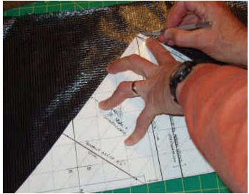
After the kite skin is cut out; open the folded kite skin, place the template on one half of the skin and put the tip of your pen through each of the holes and place a dot on the kite skin at each hole and draw a line using the cut at the wingtip, this line marks the location the bow tips.....repeat on the other side of the kite skin.....then connect the appropriate dots for identifying the batten locations, nose tape reinforcement, etc.
