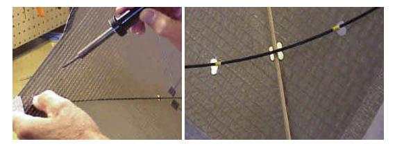
An alternate method to actually melting small holes in the kite skin, to allow the bridle to enter and exit the kite skin, is to use a large eyed needle; thread it with the bridle line and use the needle puncture the kite skin. This eliminates a larger hole in the skin of the kite. Either method works fine.
